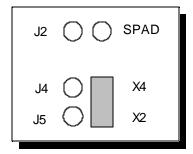
Figure 2 --- Factory default jumper configuration
